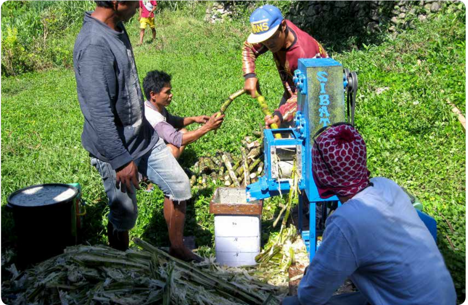
The traditional dapilan method of sugar pressing (left) is now replaced by the efficient microhydro-powered sugarcane press in some areas (above).
