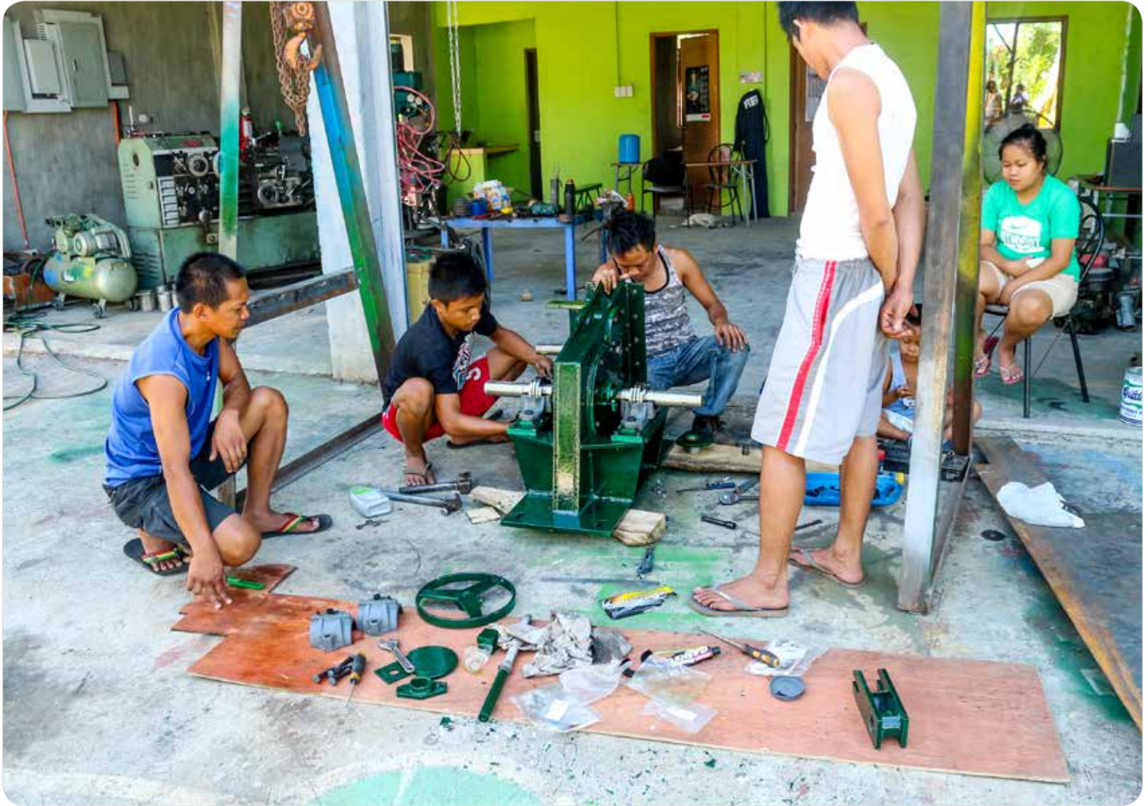
SIBAT designs and manufactures small crossflow turbines and production tools powered by microhydro in its CREATEch workshop.
