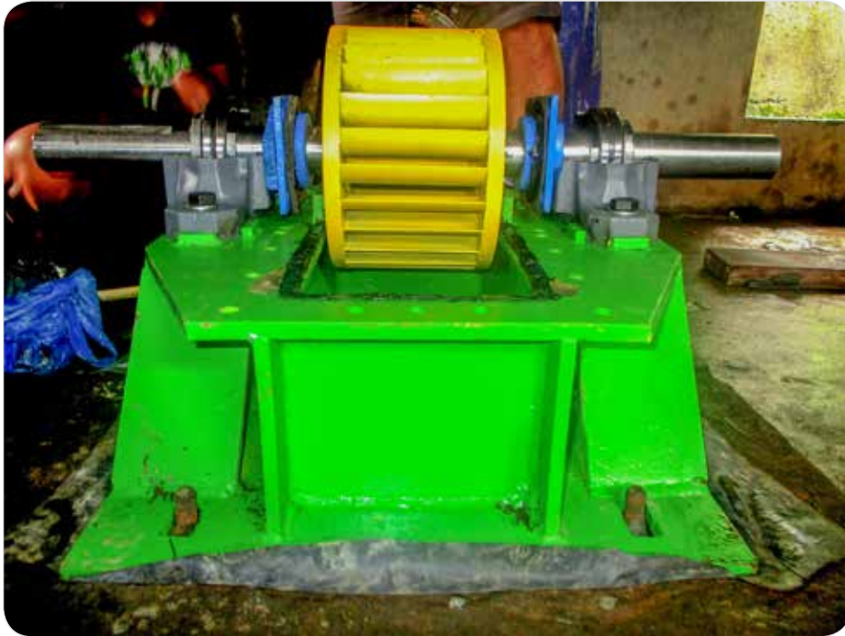
Crossflow turbine of the Balbalasang microhydro.
