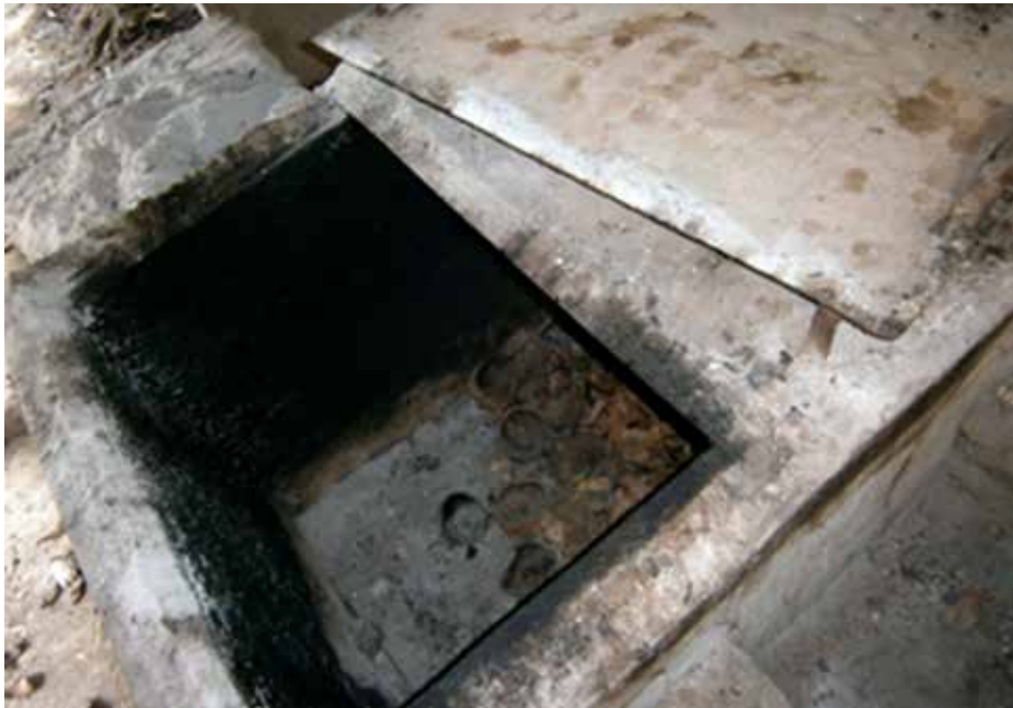
Figure 21. “Oven” component of the Mokusaku device.
